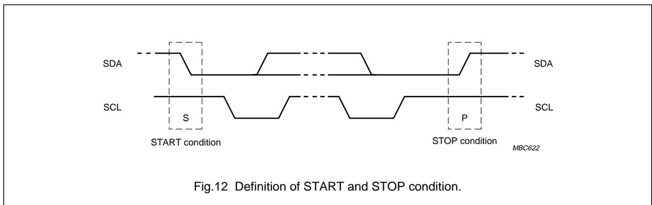
Fig.12 Definition of START and STOP condition.
