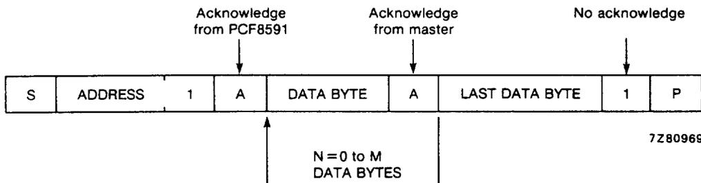
Fig.16 Bus protocol for read mode, A/D conversion.
