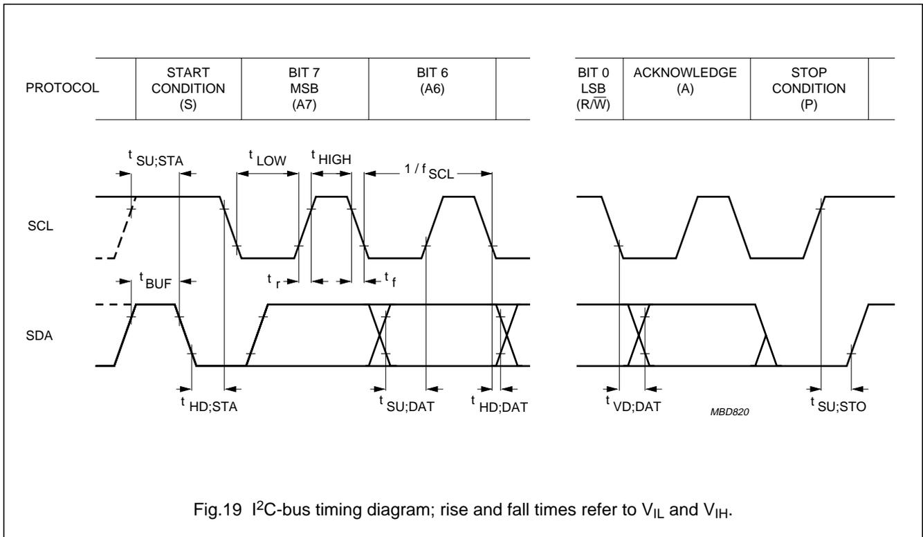
Fig.19 I<sup>2</sup>C-bus timing diagram; rise and fall times refer to  $V_{IL}$  and  $V_{IH}$ .
