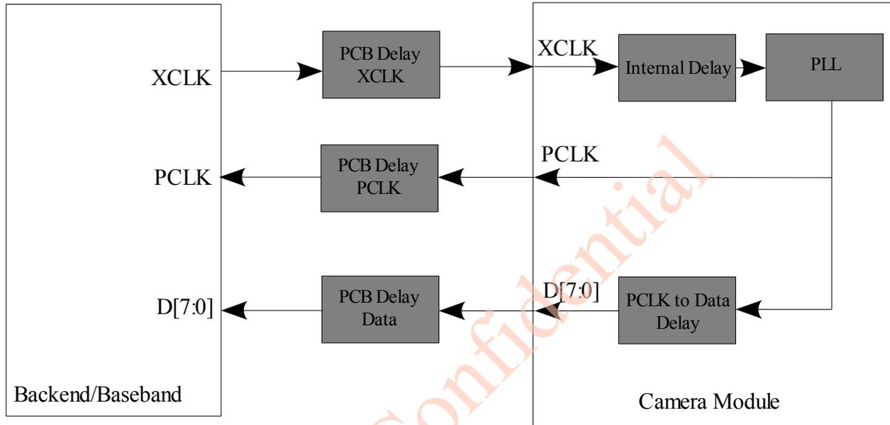
So the delay of video data to clock at backend/baseband side is very critical for timing design. If the delay is over the spec. of backend/baseband chip, the backend/baseband chip can not get video data correctly. The incorrect video data may have wrong color, fixed or moving horizontal lines.
