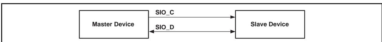
The 2-wire implementation requires one of the following two master control methods in order to facilitate the SCCB communication.
