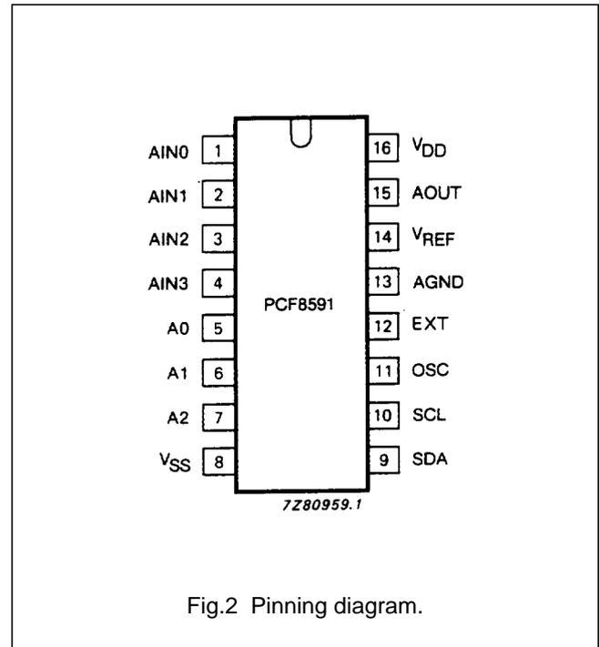
Fig.2 Pinning diagram.
