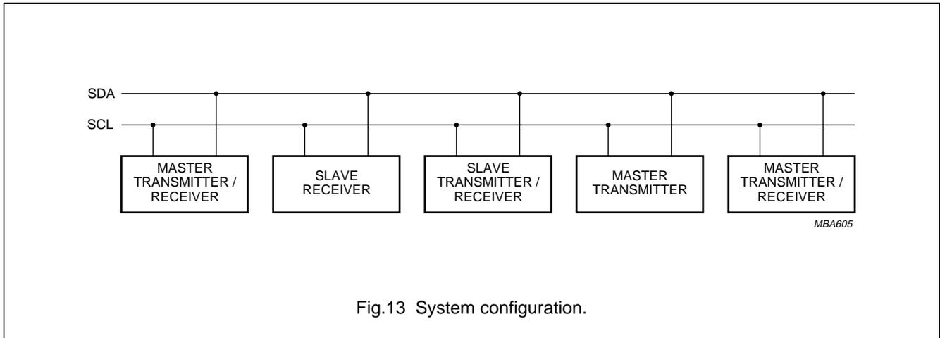
Fig.13 System configuration.
