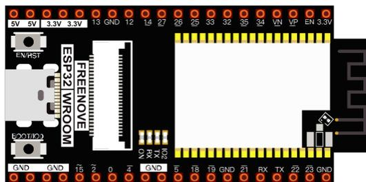
GPIO16-17 has been used to connect the integrated PSRAM on the module.
