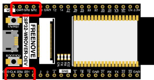
In the new release, we no longer introduce GPIO6-11.
